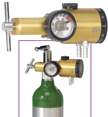
CGA-870 Yoke Inlet and DISS 1240 Outlet Connections
